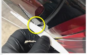
Figure 3 – Overflush greater than 1.5 mm
