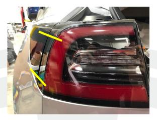
Figure 1 - Overflush check locations
